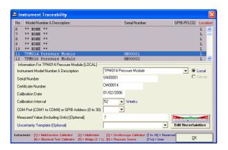
Use the Instrument Traceability function in ProSet to add the pressure modules required to the traceable list. This needs to include the scale factor of the pressure module used, eg.
