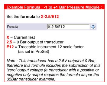
Using the **Exx** command, the scale factor is used from the central instrument traceability list as created using ProSet. When the pressure module is recalibrated the scale factor can be updated in ProSet without having to change any procedures which are using this pressure module.
