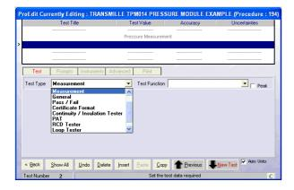
Select test function as **DC VOLTAGE** – this is selected as the signal from the transducer is a 5V DC voltage signal – this test will be configured to convert this to Bar using a scale (conversion) factor.
